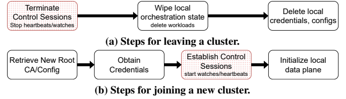
Figure 5: Showing the steps required for a node to leave an existing cluster and then join a new one. The highlighted steps are the only ones that StarLoom needs to perform since the credentials are locally available.
